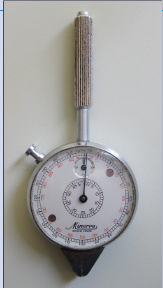
This Minerva measuring wheel, the jewel of my inheritance from my father, was used by him to measure the exact lengths of lines on blueprints and survey maps. It is a close relative of instruments used by surveyors for hundreds of years to measure the dimensions of the Earth.
